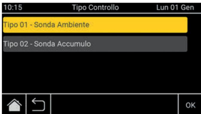
In the "Probe Management" menu, the input type can be configured.
