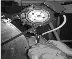
If the measured distance is higher or lower, it's necessary to tight or to release the belt by using the apposite screw.
