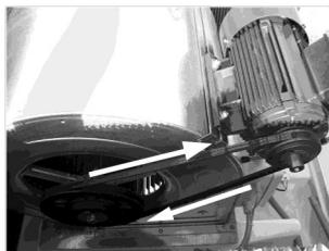
4. If the fan should rotate in the wrong direction, it's necessary change the main switch power supply connections by exchanging L1 and L2 connections
