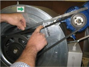
Place a perfectly straight extruded bar on the two pulleys, by using a finger apply a light force on the middle of the belt and measure the distance between the flexed belt point and the bar. The distance should be between 1cm and 1,5cm.
